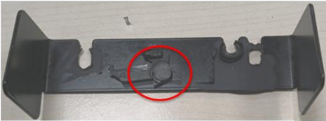
Figure 1: Example of excessive sealant that can block the membrane.
