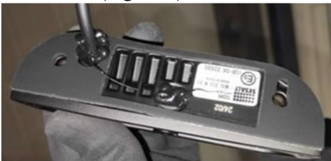
Figure 2: Incorrect Installation. The vents for the condensation membrane are blocked by excess sealant.
